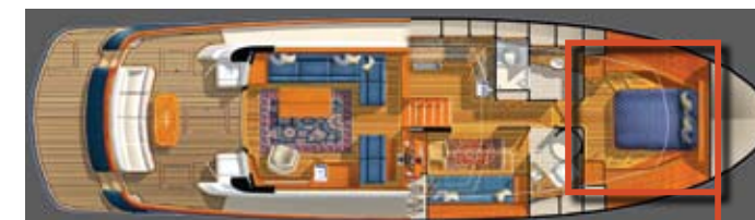
UNLIKE PRICE’S CUSTOM DESIGN, THE STANDARD LAYOUT INCLUDES AN AFT-FACING BERTH IN THE MASTER STATEROOM.
