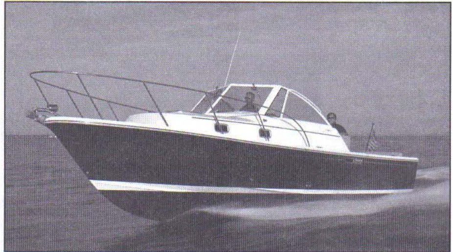
Above: A gently sloping sheer, high windshield and trunk cabin are all marks of a New England-style boat. The Surfhunter 29 has them all. Note the bow's narrow forefoot and sharp entry.
